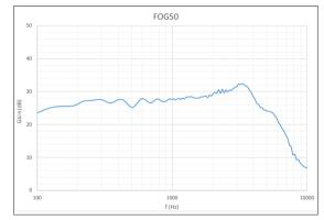
Figure 2: Nominal frequency response curve as measured in a 2 cc coupler.
